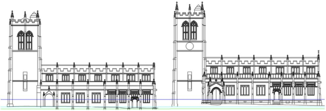
*This drawing shows the South side of the church before and after with the 1795 flood line on both. An extra 7 feet was added to the tower.*
