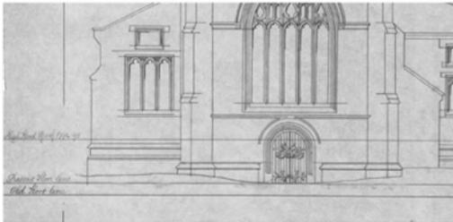
*This drawing shows the extent of the problem. The bottom line shows the earlier floor level but by 1780 it had been raised to be level with the bottom of West end door.*
